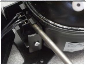
To install new module: Push the 3-prong plug evenly onto the compressor. Hook the module onto the back of the bracket first and then snap into place. Turn the Philips head screw counter clockwise to secure the module. Replace (PCB Board) and the wires to their original locations on the module.
